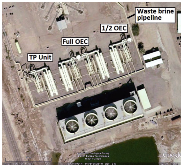
Fig. 17.8 Gould I bottoming binary units installed just south of the Heber 1 double-flash plant: Google Earth image, Feb. 1, 2008, labels by author [WWW].
