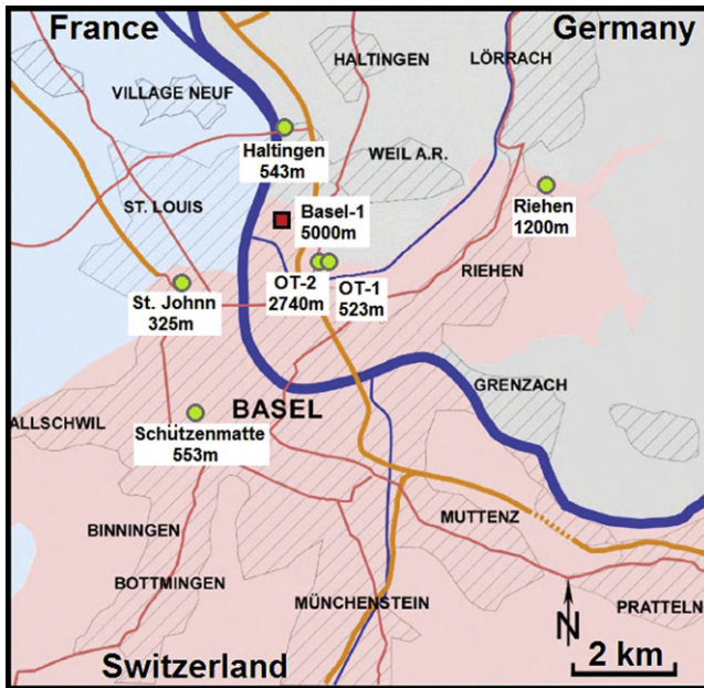
Figure 22.24 Well field at Basel: the circles are monitoring wells showing the depth of sondes [24] [WWW].
