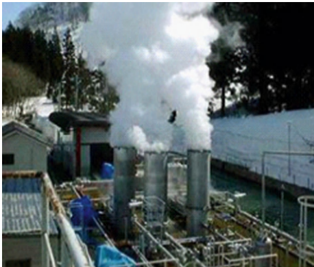
Figure 22.6 HDR research facility at Hijiori, Japan. Silencers at the production well during a 2-year circulation test, 2000–2002 are shown. The reservoir lies at a depth of 2300 m, with a temperature of 270°C [11].
