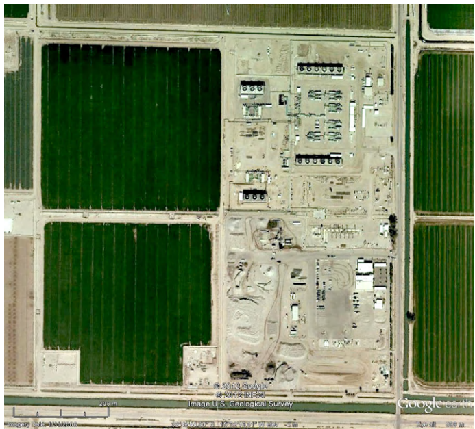
Figure 23.4 Aerial view of the Heber 2 binary plant near Heber, CA [18]. The 10 MW Gould II unit (with a 3-cell cooling tower) lies just west of the original SIGC plant. Heber South is just south of Gould II; see Fig. 17.6. Google Earth image from 1-31-2008 [WWW].
