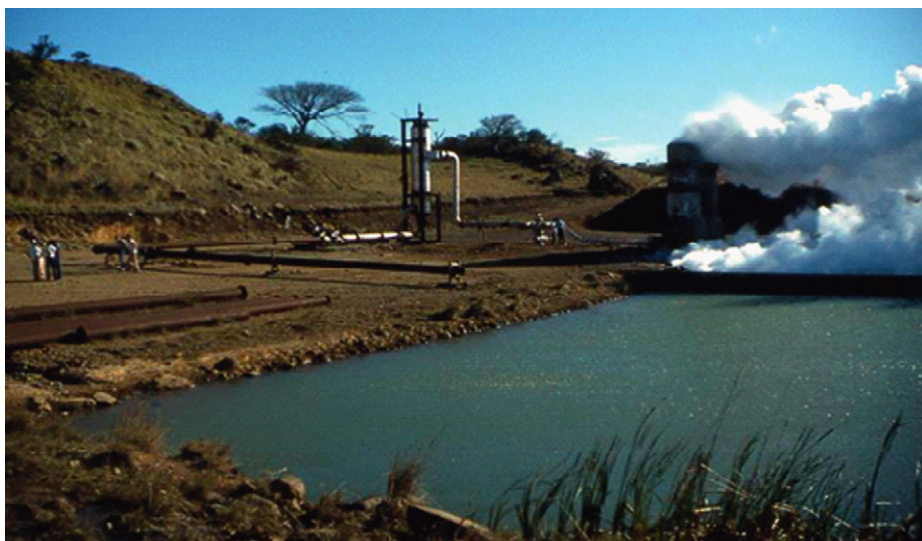
Fig. 16.14 Flow testing the discovery well at Miravalles, PGM-01. Photo by author [WWW].
